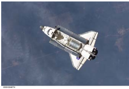
ISS013-E-48774 --- Discovery approaches ISS for docking with Leonardo Multipurpose Logistics Module (MPLM) in the payload bay.
