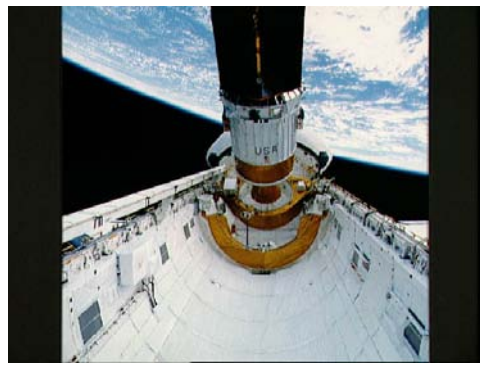
STS029-71-000AE---IUS/TDRS-D deployment from Discovery payload bay.
