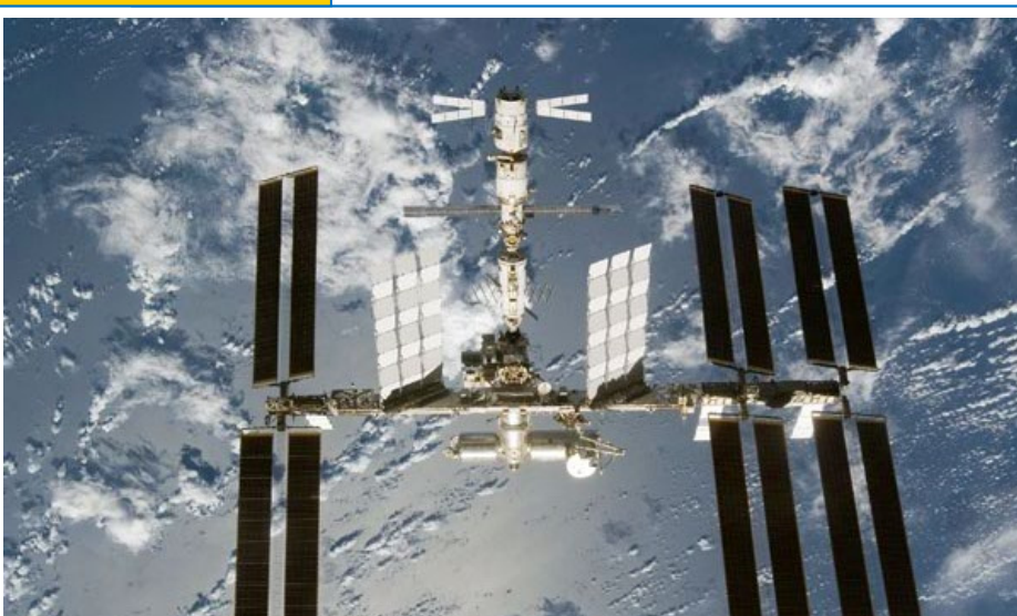
ABOVE: S124-E-009982 (11 June 2008) --- View of ISS configuration post Shuttle sep shows Kibo attached to Harmony at bottom center with first ESA ATV Docked at top center. AT LEFT: S124-E-010186 --- The Kibo laboratory (center left) is shown after attachment to port side of Harmony Node with: Kibo logistics module at bottom left, Columbus lab at center right, and at top center is Dextre along with two docked Russian spacecrafts.
