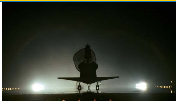
STS096-(S)-010 --- First flight of Functional Drag Chute with strengthened door pins after STS-95 problem (door fell off at SSME throttle-up). Inconel replaced aluminum pins.
