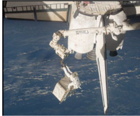
S135-E-007515 --- With his feet secured on a restraint on the ISS robotic arm or Canadarm2, Ron Garan/ Exp 28 Flight Engineer, carries the pump module,
