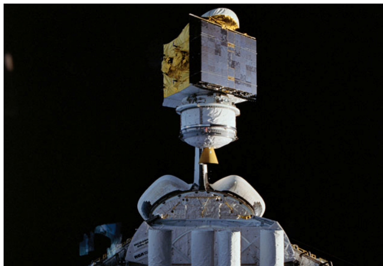
ABOVE: 61C-005-0036 -- SATCOM Ku-1 Communications Satellite deployed from Columbia. BELOW: 61C-S-050 (18 January 1986) --- Second Shuttle night landing. View is of the Shuttle's main landing gear touching down at EAFB with streams of light trailing behind the orbiter.
