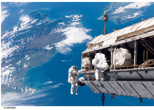
LEFT: S116-e-05983 - Curbeam (left) and Fuglesang conduct EVA1 tasks for installation of P5 Truss. New Zealand and Cook Strait are seen in the background.
