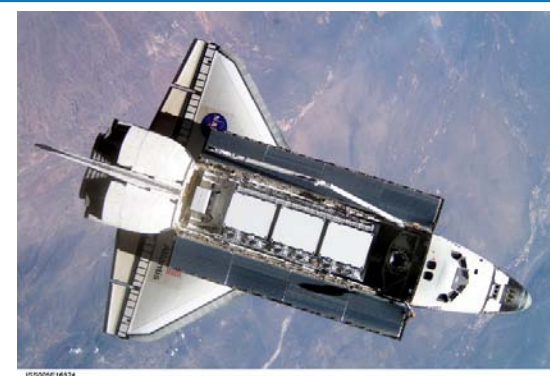
ISS005-E-16524 --- Atlantis on approach to ISS for rendezvous and docking operations to deliver the 15 ton S1 Truss.
